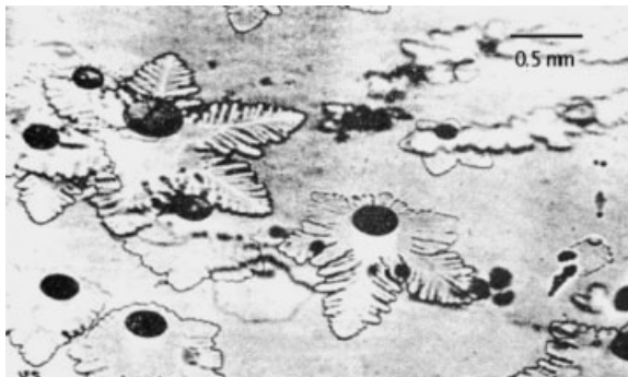
Figure 14.5 Tyndall figures: dendritic melting of ice.
