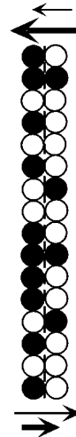
Figure 22.2 Schematic of compositions and transition rates at the interface. The lengths of the heavy and light arrows indicate the transformation rates of the black and white atoms, respectively.
