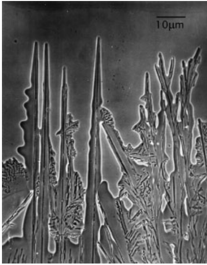
Figure 27.8 Transparent alloy, succinonitrile-borneol, which resembles the aluminum-silicon alloy.
