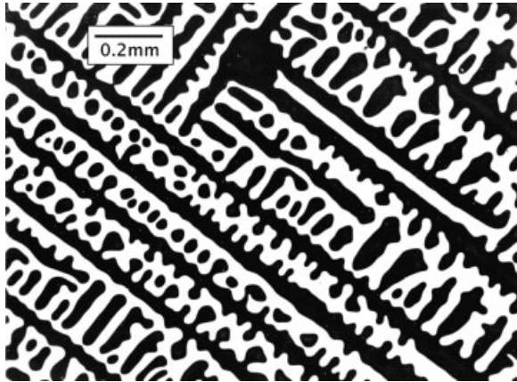
Figure 28.3 During coarsening, the arms can become detached from the main stem of the dendrite.
