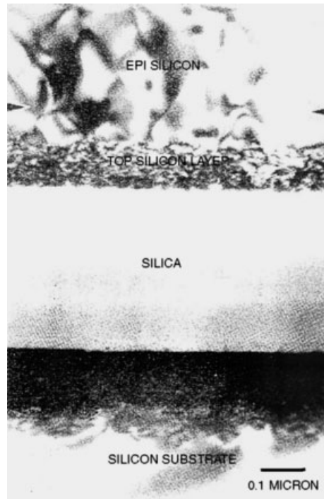
Figure 6.15 SIMOX silicon-on-insulator. (After Pinizzotto [6]).
