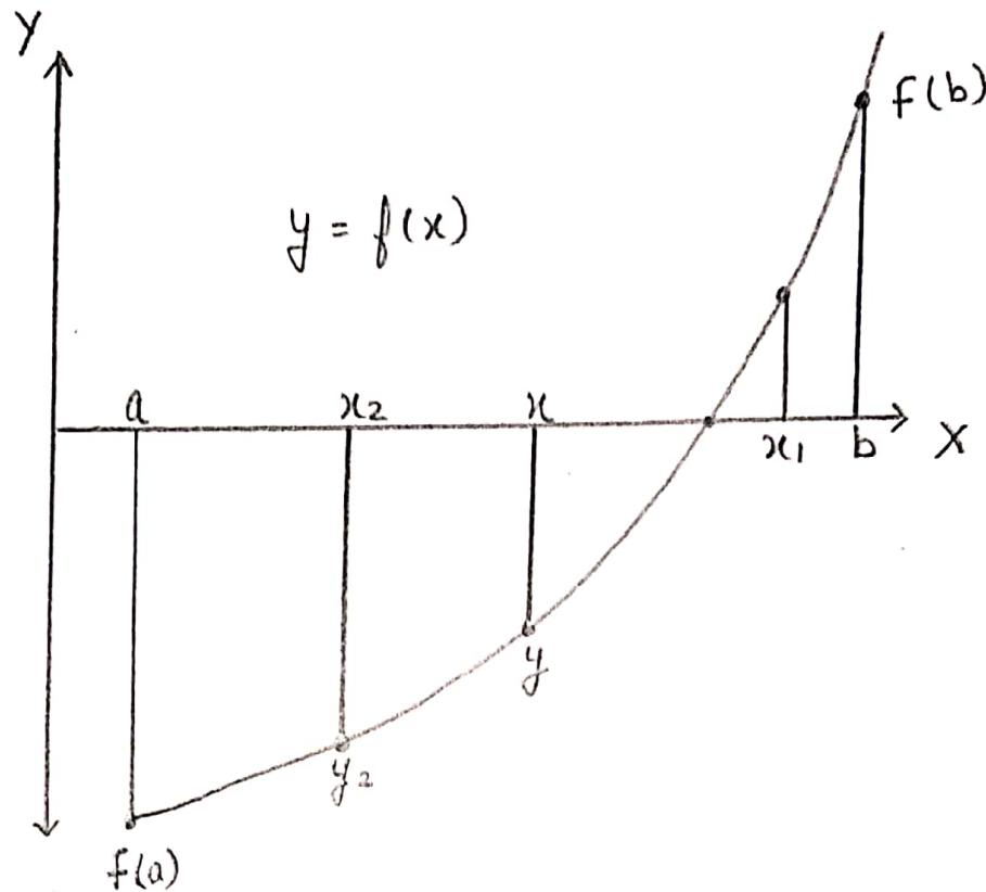
Geometrical Construction of Iterative Method
