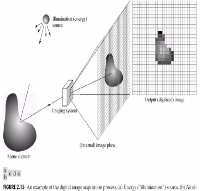
FIGURE 2.15 An example of the digital image acquisition process. (a) Energy ("illumination") source. (b) An el-ement of a scene. (c) Imaging system. (d) Projection of the scene onto the image plane. (e) Digitized image.
