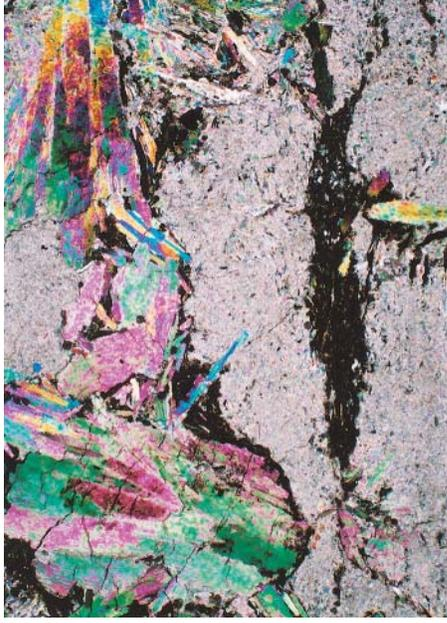
**(b)** Anhydrite and secondary gypsum: small crystals and laths of anhydrite (bright colours) being replaced by large, low birefringence, porphyrotropic gypsum crystals. Crossed polars. Permian (Zechstein). Teesside, England. Field of view 6 × 4 mm.
