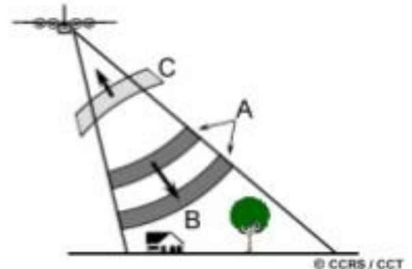
*By measuring the time delay between the transmission of a pulse and the reception of the backscattered "echo" from different targets, their distance from the radar and thus their location can be determined*
