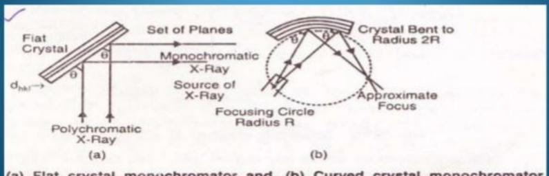
(a) Flat crystal monochromator and, (b) Curved crystal monochromator.
