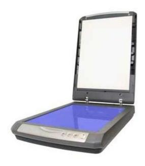
Scanner captures images from the source which are then converted into a digital form that can be stored on the disk. These images can be edited before they are printed.
