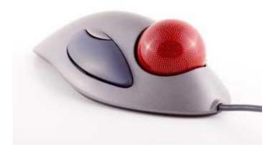
Since the whole device is not moved, a track ball requires less space than a mouse. A track ball comes in various shapes like a ball, a button, or a square.
