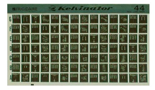
Ultra-fiche:- Ultra fiche is another form of microfiche which contains about 2000-3000 pages having high reduction ratio exceeding 90x. Ultra fiche is not in common use. Aperture Cards:- An aperture card is an opaque tab card with 4 rectangular hole or holes designed for mounting or insertion of microfilm. The card can also contain key-punched, interpreted and printed information for identification and retrieval. It is an united medium useful for engineering drawings system.
